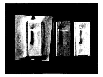
*Fig. 7. Example of milled panel formwork, vacuum formed panel, and cut final panel.*
