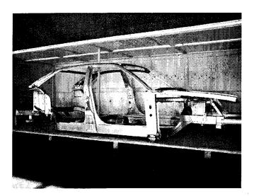
Fig. 2. The Audi A8 frame, showing the relationship between surface and structure.
